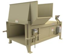
Compact dry waste material and cardboard for recycling. They can be supplied with a variety of feed configurations including ground level, chute, hopper, deck and offset. They are ideal for use at manufacturing facilities, multi-story hotels, office and commercial buildings, big box retailers, warehouses, and distribution & fulfillment centers.
